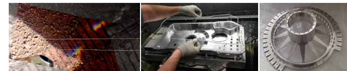
Nahaufnahme des Marsbodens von Nasa/JPL Mars Exploration Rover Opportunity; ALD: Fit-Check einer Dichtung für die Ultra-clean Zone; das PSHS-Karussell führt Proben Analyse-Instrumenten zu / Close-up view of Martian terrain by Nasa/JPL Mars Exploration Rover Opportunity; fit-check of a seal for the ultra-clean zone; PSHS-carousel for transportation of samples to analysis instruments
